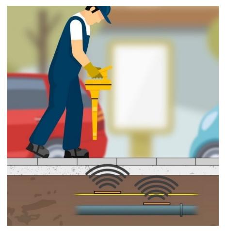
The use of RFID technology allows the precise location of the buried sensor with the TRENCHIP reader.
